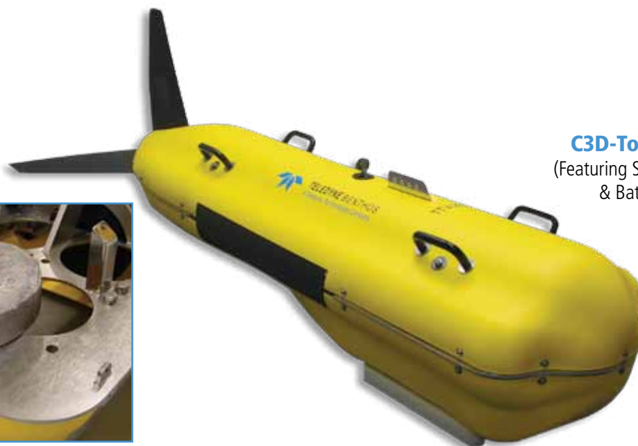
Dummy weight installed in bow of C3D Tow Vehicle
