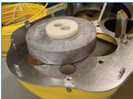
Dummy weight installed in bow of C3D Tow Vehicle
