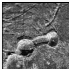
2D side scan and bathymetry of impressions of oil rig footings
