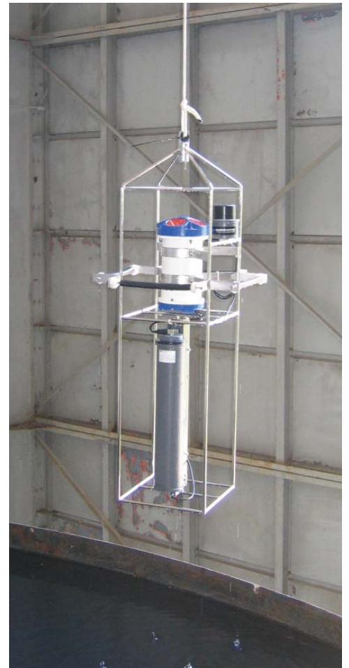
Figure 1 ADCP with SR-50 below and remote transducer head mounted in the upper right section of the frame
