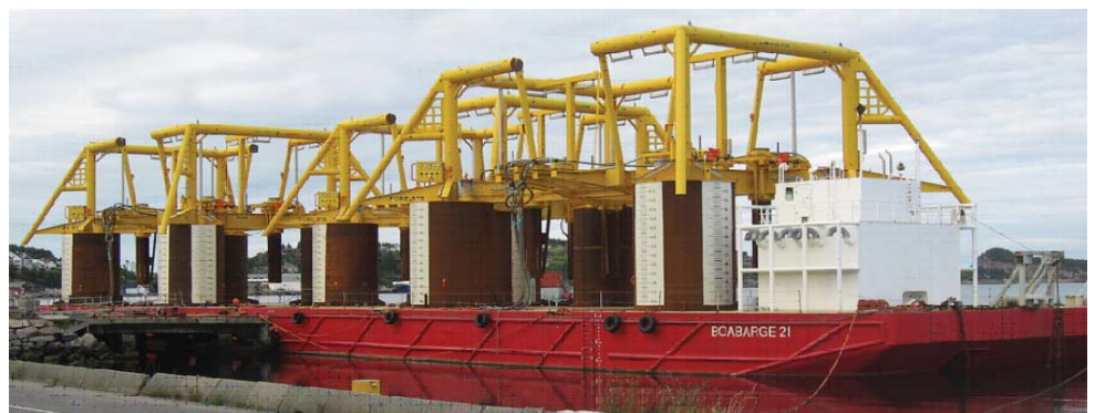
Figure 1 Barge used to deploy subsea structures
